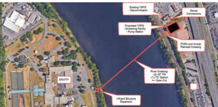
Figure 1 - Aerial photograph of the project area indicating major elements of the LTCP/IWP Phase 2 project
